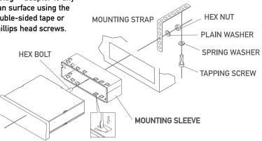
TYPICAL FRONT-LOAD DIN MOUNTING METHOD
